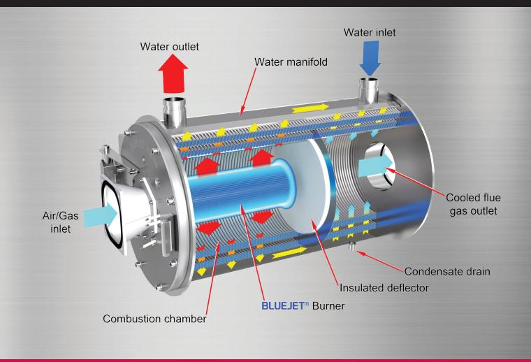
Torus' Bluejet<sup>®</sup> burner offers industry leading modulation capacity, flame retention and combustion quality. Whether natural gas or LP gas, BlueJet's low NOx design works in perfect concert with our Tru-Flow fuel/air system providing consistent reliable operation.
